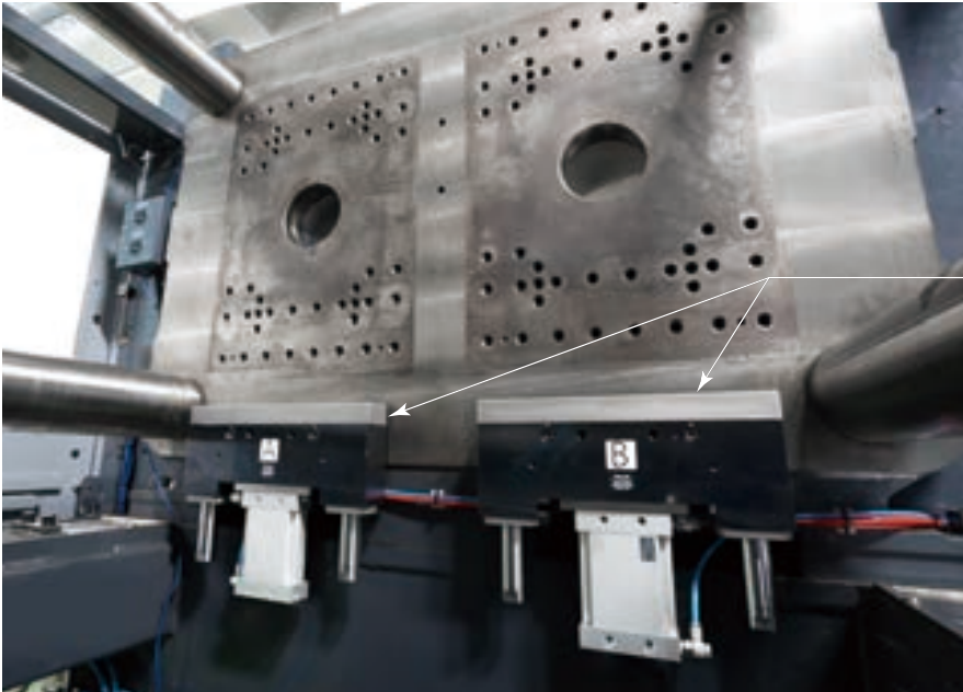
2,800kN (280ton) Two-color IMM Die leveler
