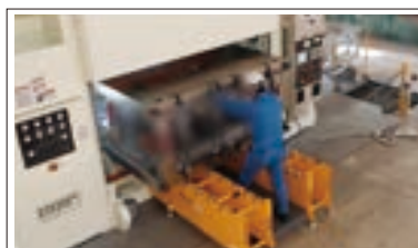
20,000kN press machine 8ton The loding/unloaidng of die
