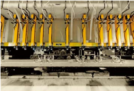
34,000kN(3,400tonf) Transfer press
