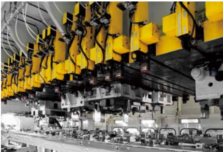
23,000kN(2,300tonf) Transfer press
