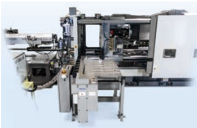
Die changer Powered, Pusher type Fixed roller table Number of load 1die
