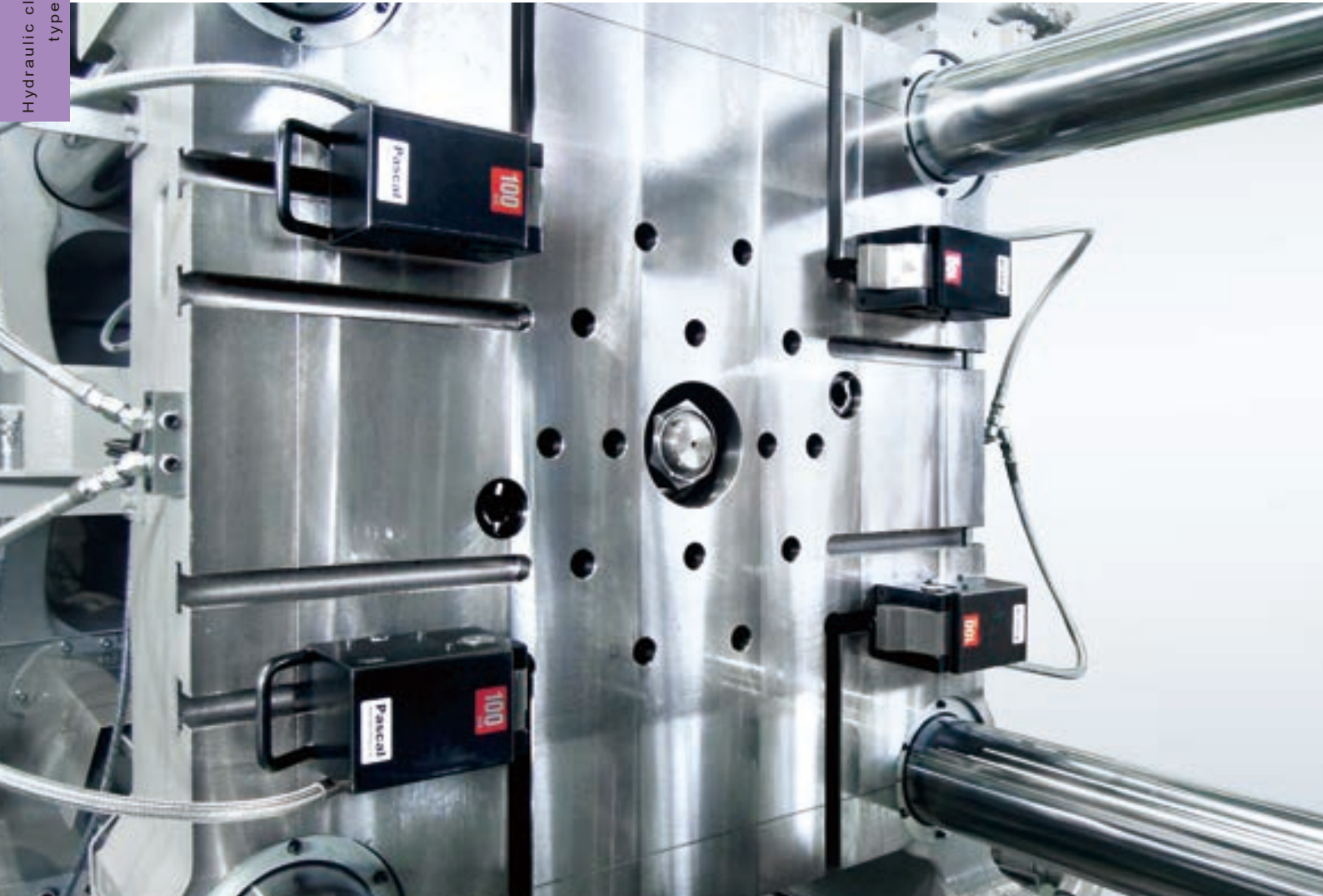
5,000kN (500ton) Die-casting machine Hydraulic clamp, slidable type TYB
