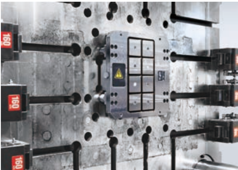
8,500kN (850ton) Die-casting machine C-plate mag clamp & Hydraulic clamp TYB
