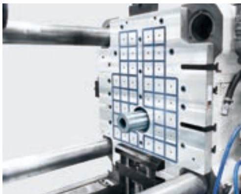
3,500kN (350ton) Die-casting machine Mag clamp fixed side
