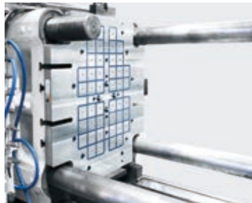
3,500kN (350ton) Die-casting machine Mag clamp movable side
