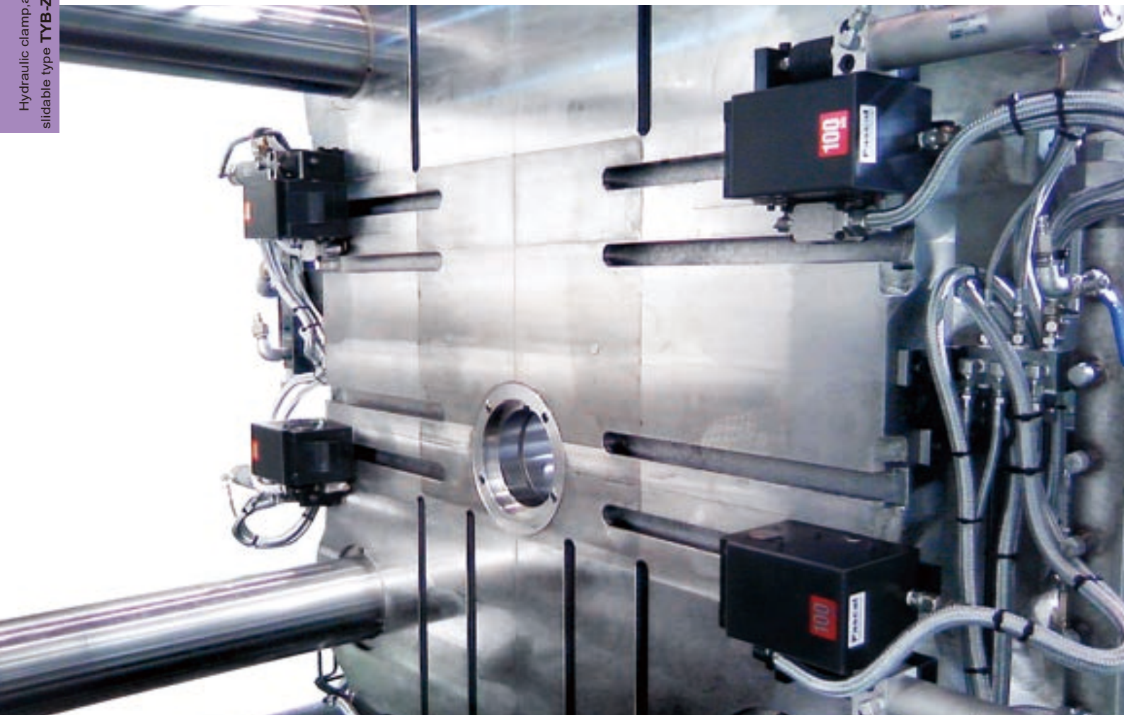
6,500kN (650ton) Die-casting machine Hydraulic clamp, automatic slidable type TYB-Z
