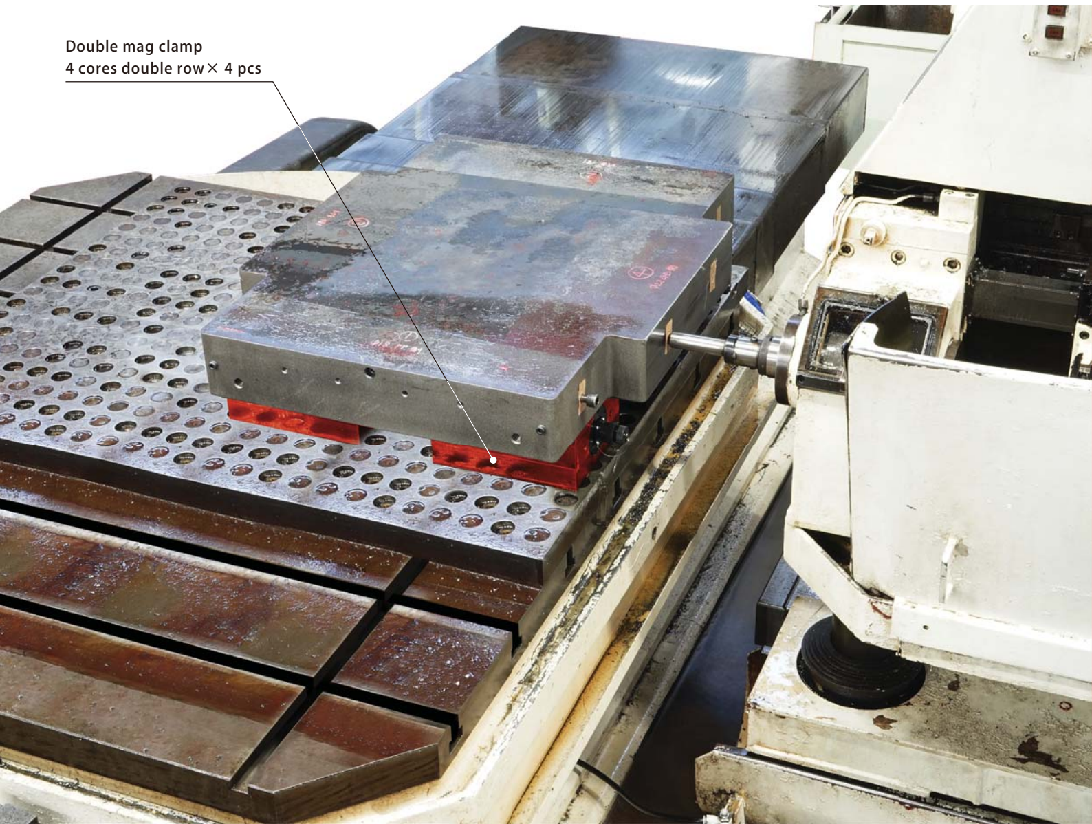
Double mag clamp 4 cores double row × 4 pcs Total clamping force on single side 117.6kN
