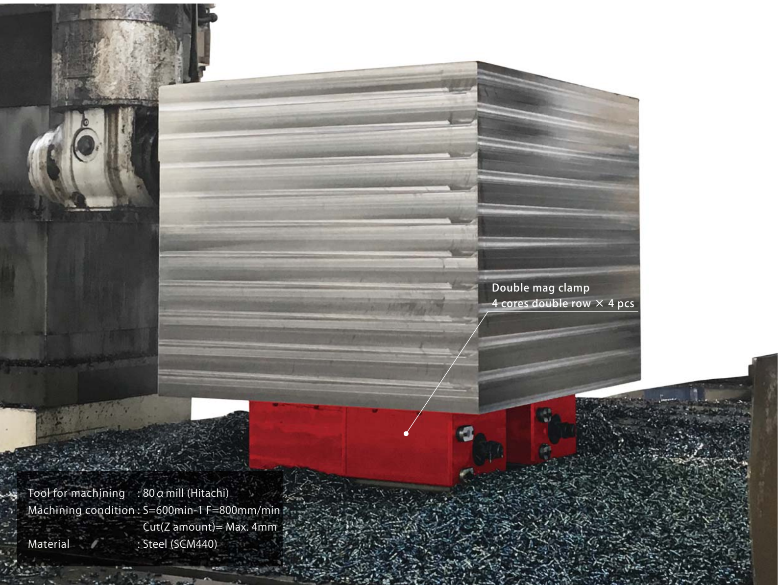
Double mag clamp 4 cores double row x 4 pcs Total clamping force on single side 117.6kN
