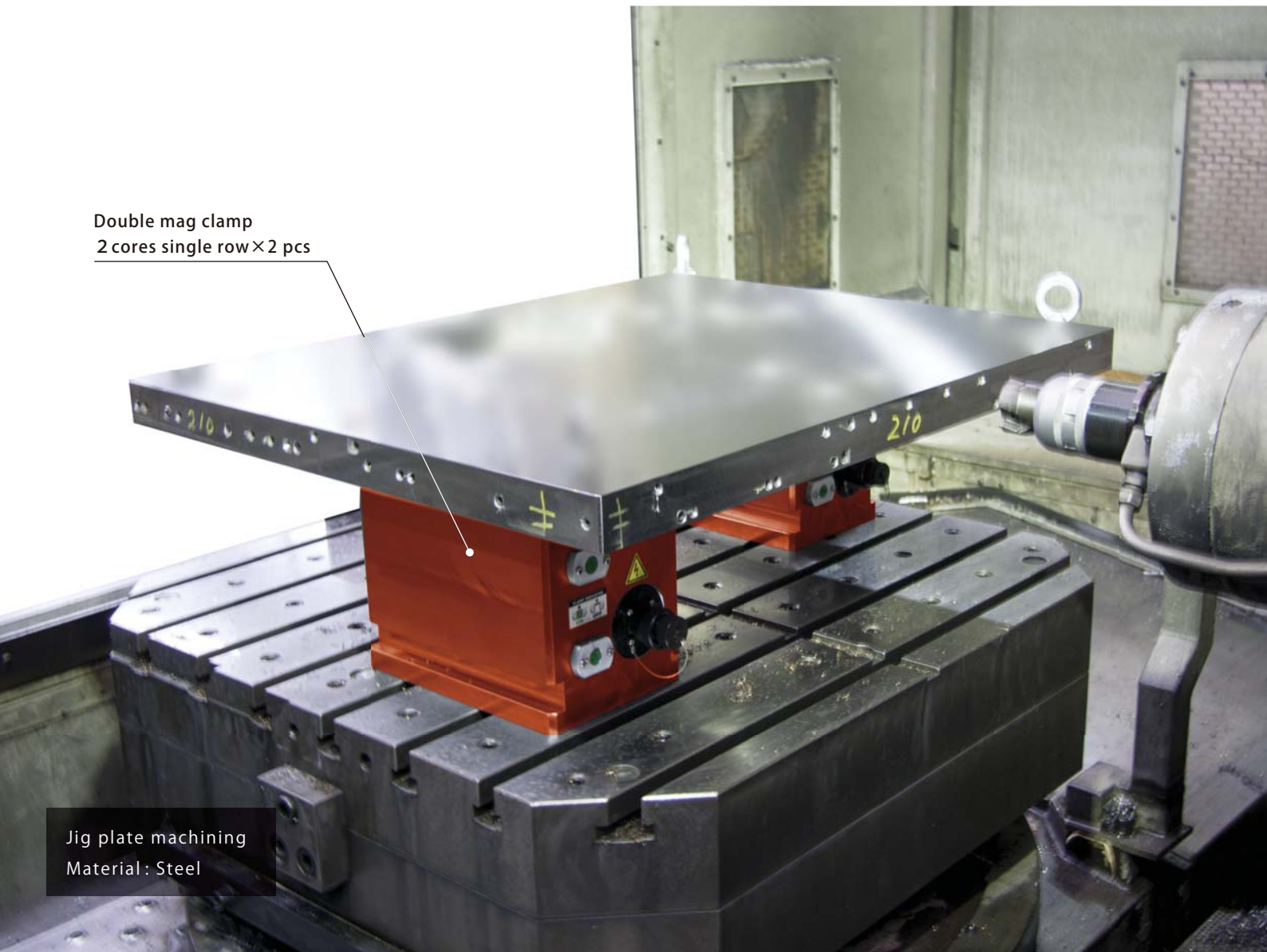
Double mag clamp Double cores single row × 2 pcs Total clamping force on single side 29.4kN
