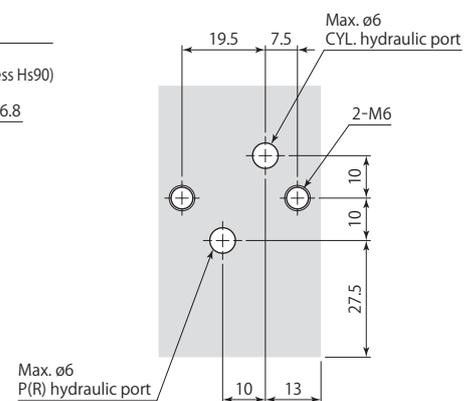
For manifold piping, the mounting surface finish must be no rougher than Rz6.3 (ISO4287:1997).
