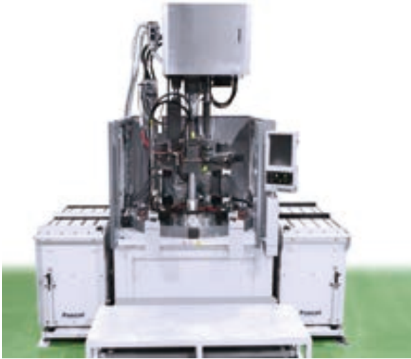
1,500 kN IMM Mold 800kg × 2 molds × 2 Mold changer: Manual, Non track
