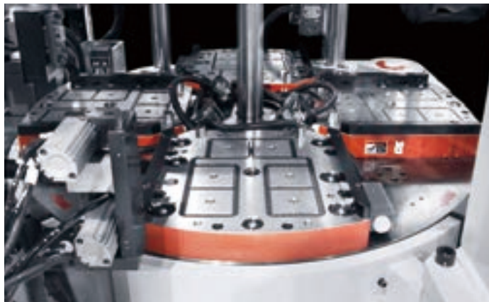
450kN (45ton) Vertical IMM (rotary) Mag clamp for lower mold
