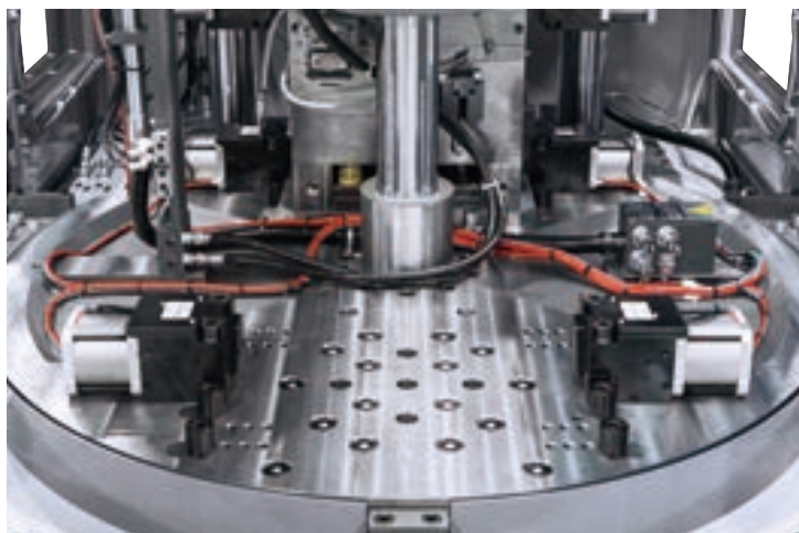
1,500kN vertical IMM Air clamp TLA
