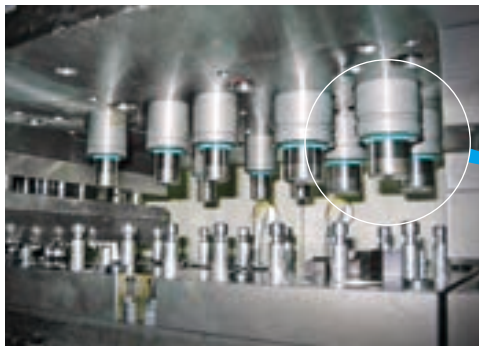
4,000kN (400tonf) Progressive press upper Mini N2 gas spring adopted example
