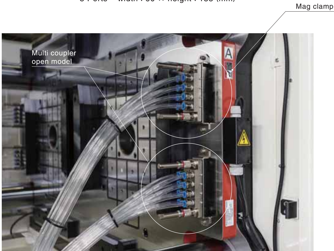
For temperature control & air valve gate
