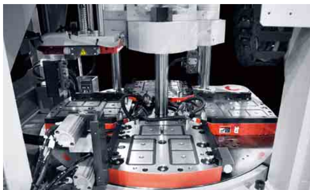
400kN (40ton) Vertical Rotary IMM Magnet clamp
