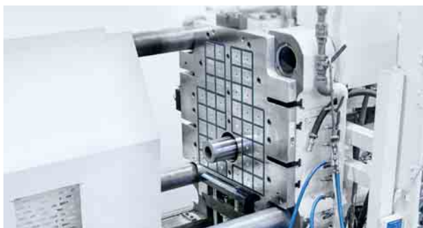
3,500kN (350ton) Magnetic clamp for diecasting machine
