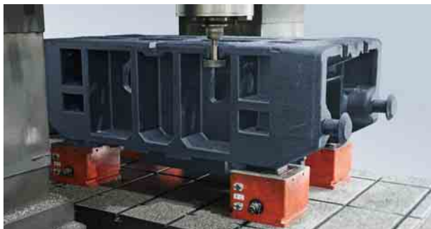
Die machining with double mag clamp (dual side magnet)
