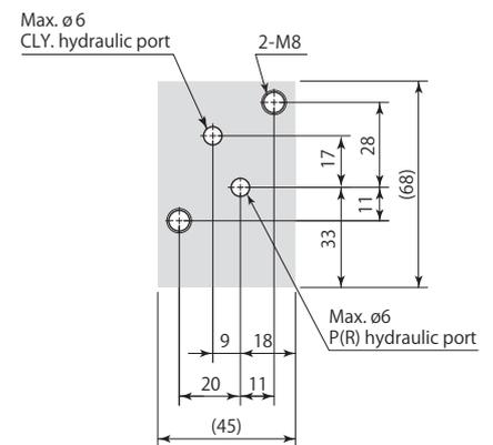
For manifold piping, the mounting surface finish must be no rougher than Rz6.3 (ISO4287:1997).
