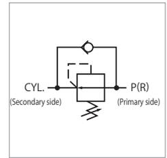
Internal hydraulic pressure of circuit can be partially reduced. This is a non-leak type that requires no drain.
