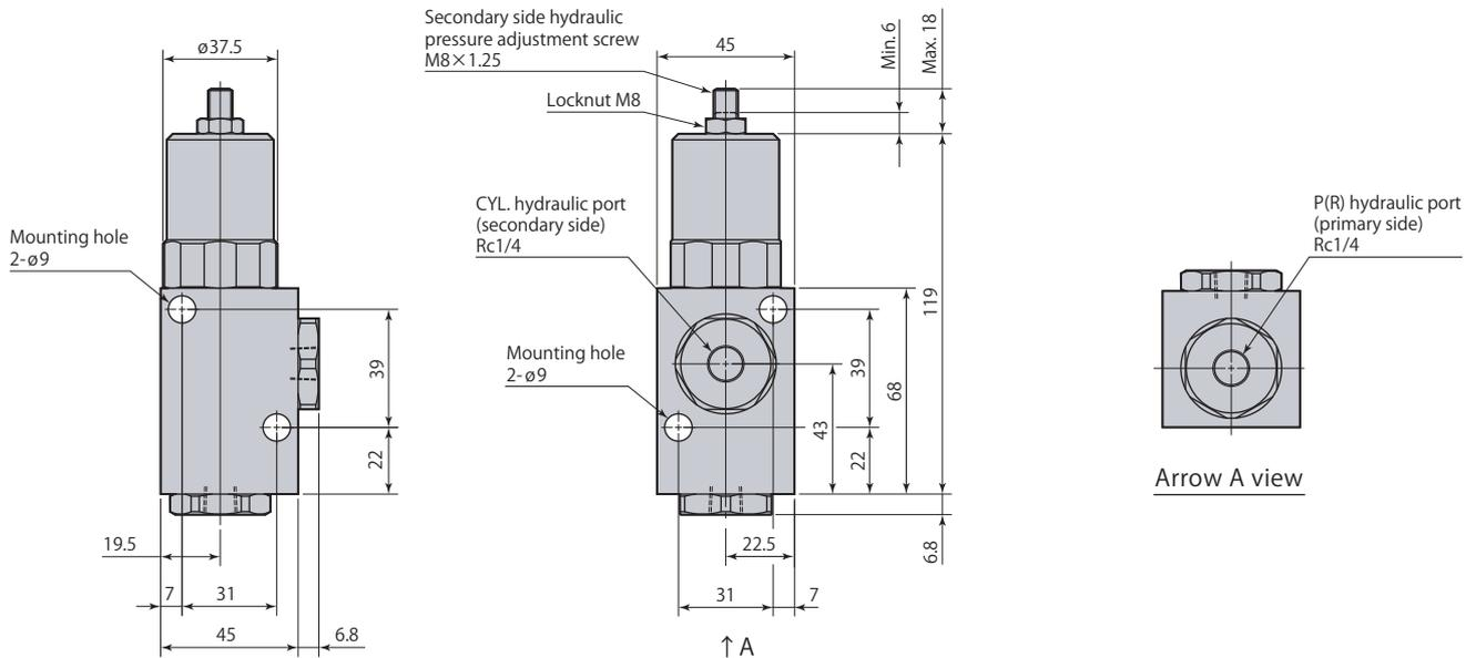
**VRG-□S** VHD linking \*With internal filter (P & CYL. hydraulic ports)
