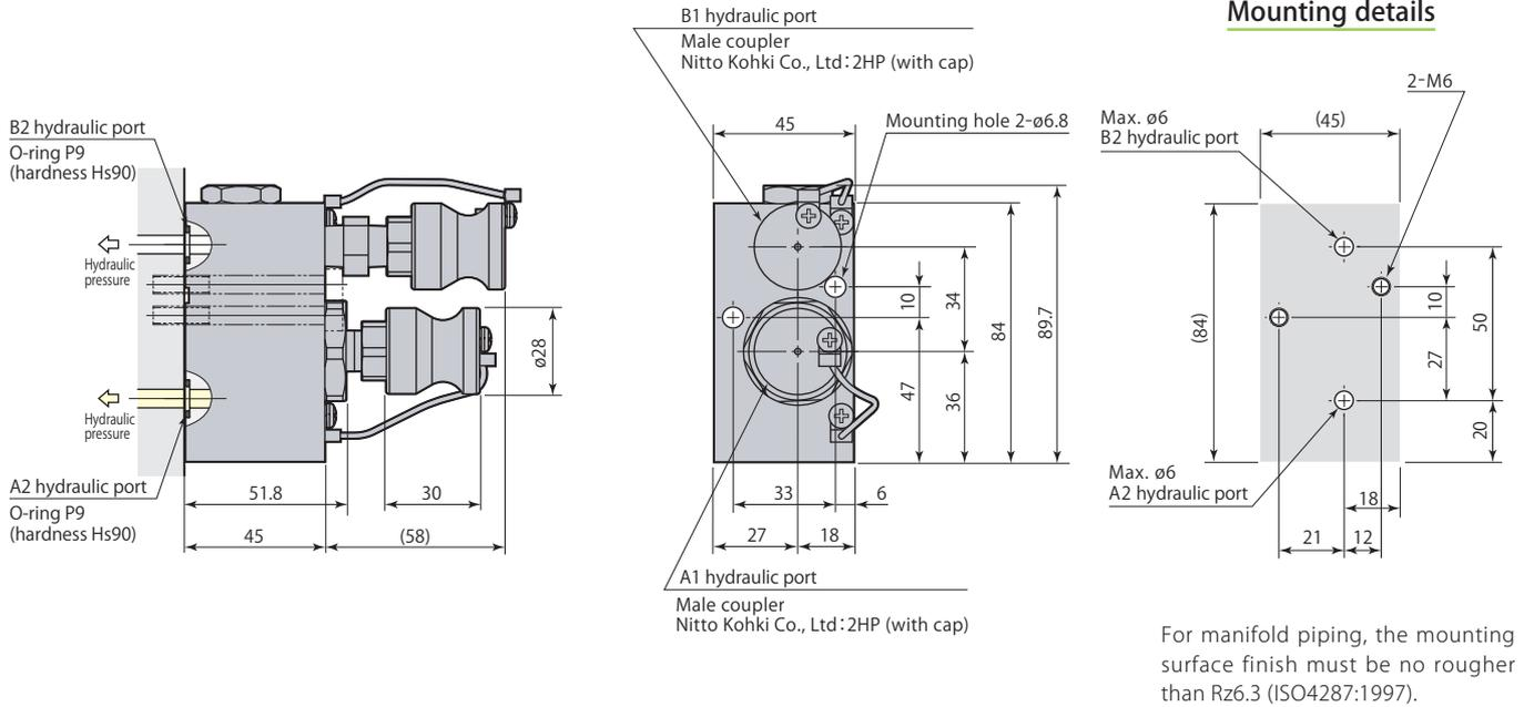
**VCB-HT** Piping mounting \*With internal filter (A1 & A2 hydraulic ports)
