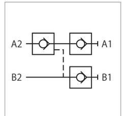
This is a non-leak valve, with which coupling of double acting clamp can be performed easily and clamping circuit pressure can be retained over a long period of time after disengagement of hydraulic pressure source.
