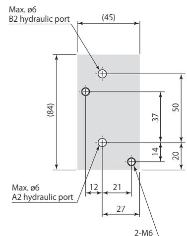
For manifold piping, the mounting surface finish must be no rougher than Rz6.3 (ISO4287:1997).
