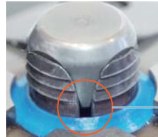
4 Grippers (Old model) Air blow model Open space where metal chips can intrude is created during clamping.
