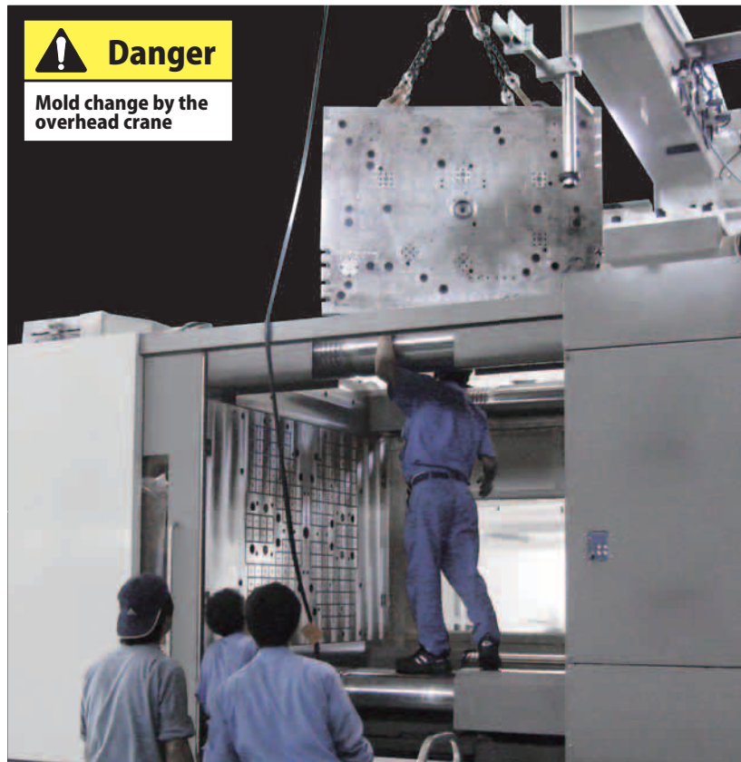
Carelessly coming under the craned mold.
