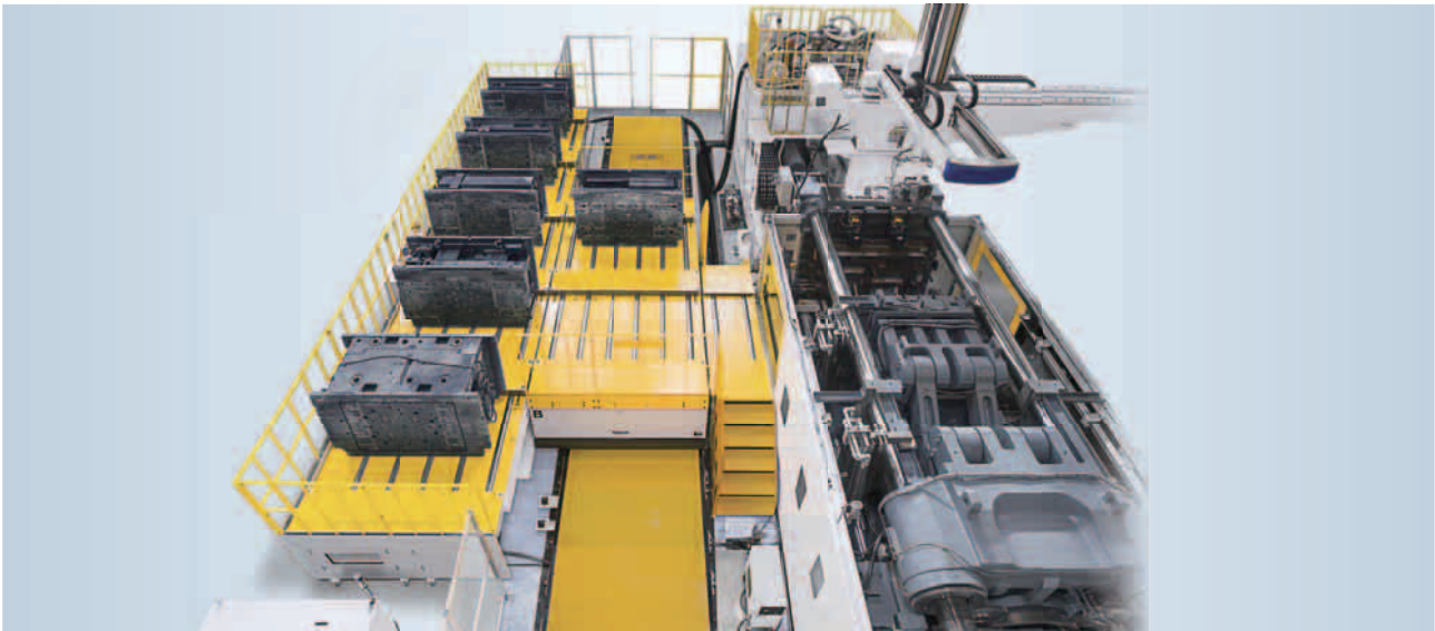
12,700kN (1270ton) IMM Horizontal loading Mold changer : Powered, Drive rollers type
