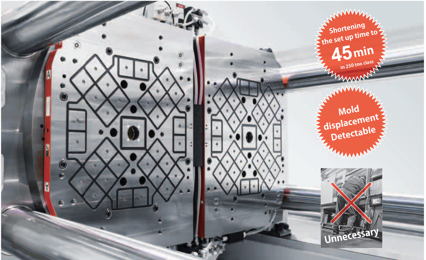
6,000kN (600ton) Two-color IMM Vertical loading Mag clamp
