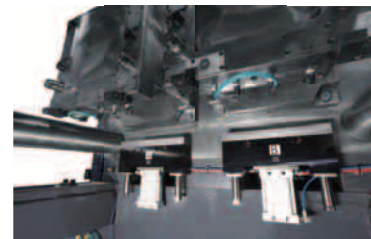
2,800kN (280ton) Two-color IMM Die leveler
