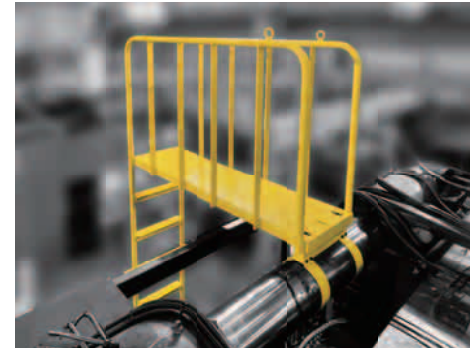
Safe working space is guarded by handrails
