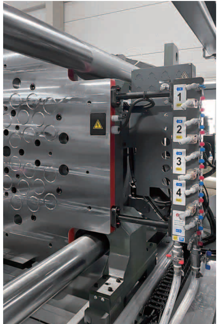
3,500kN (350ton) IMM New valve stand horizontal connection model
