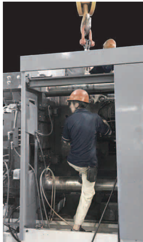
Unhooking the mold stepping on the machine tie bar.
