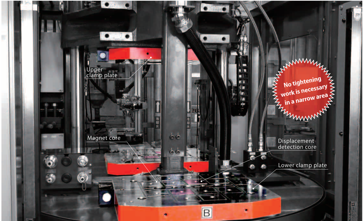
750kN (75ton) Vertical IMM (fixed table)
