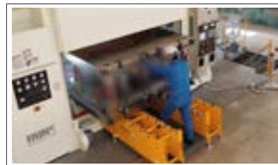
20,000kN press machine 8ton The loding/unloadng of die
