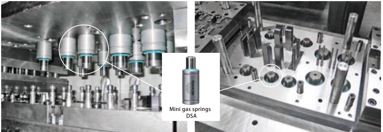
4,000kN (400tonf) Progressive press mini gas spring model DSA Adopted example (photo left : upper, right : lower)
