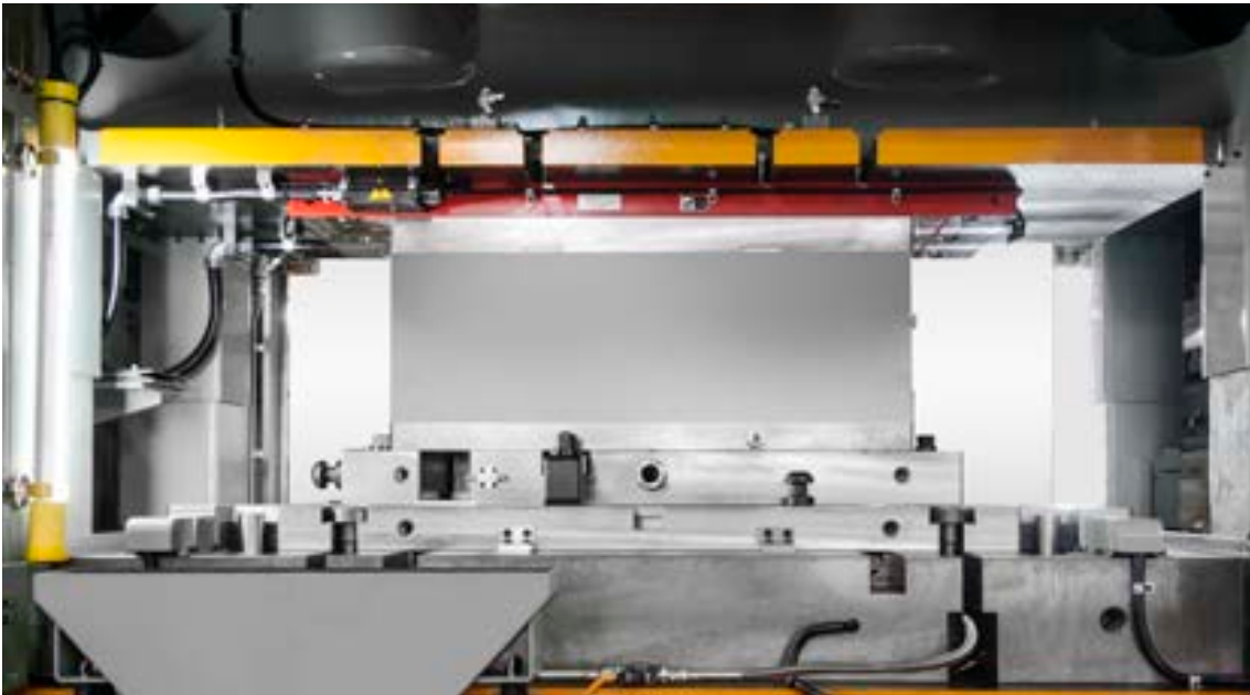
2,000kN (200tonf) High velocity press machine press mag clamp
