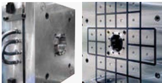
1,800kN (180ton) IMM vertical loading Octagonal locate ring & Mag clamp
