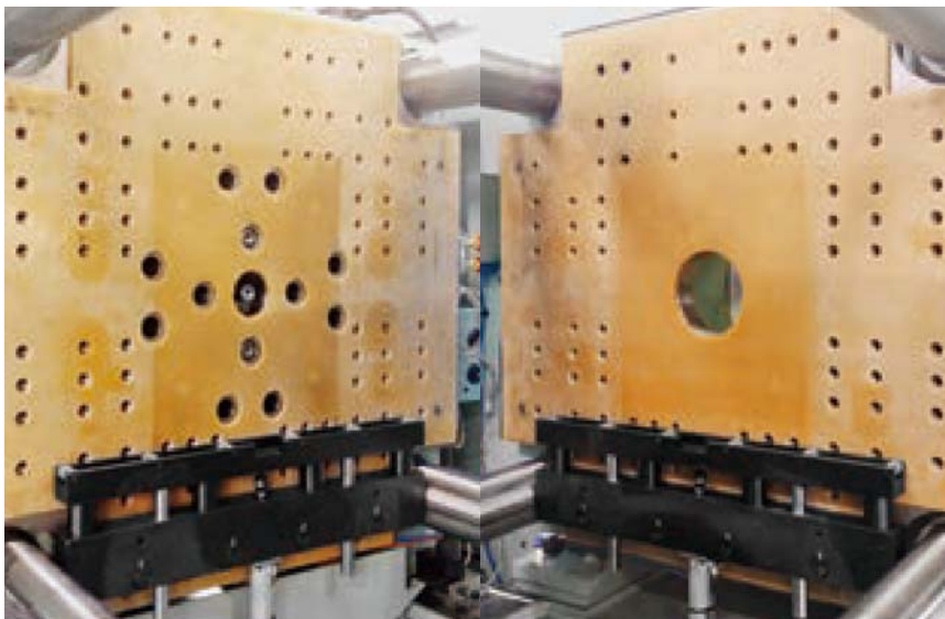
3,500kN (350ton) IMM horizontal loading Die setting roller
