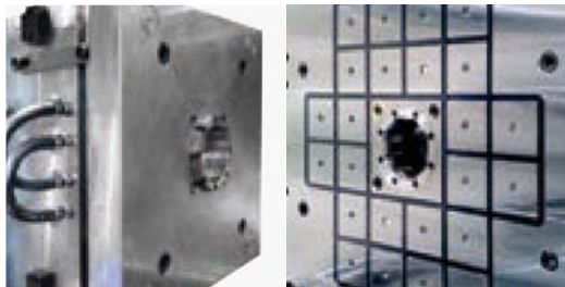
1,800kN (180ton) IMM vertical loading Octagonal locate ring & Mag clamp
