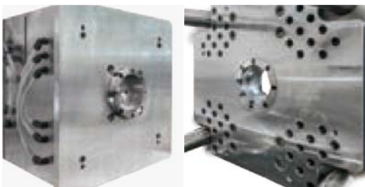
500kN (50ton) IMM vertical loading Octagonal locate ring
