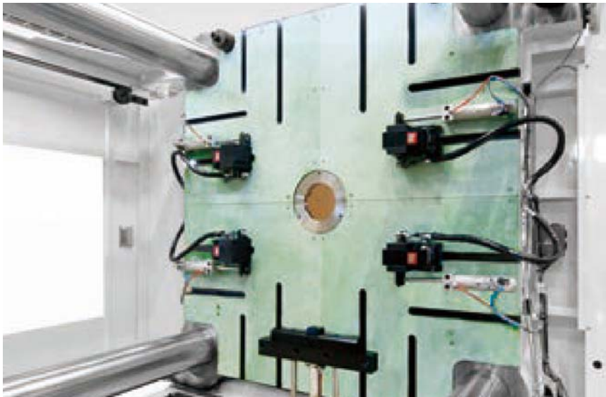
6,500kN (650ton) IMM vertical loading Die setting system & Hydraulic clamp, automatic slidable type TYC100Z
