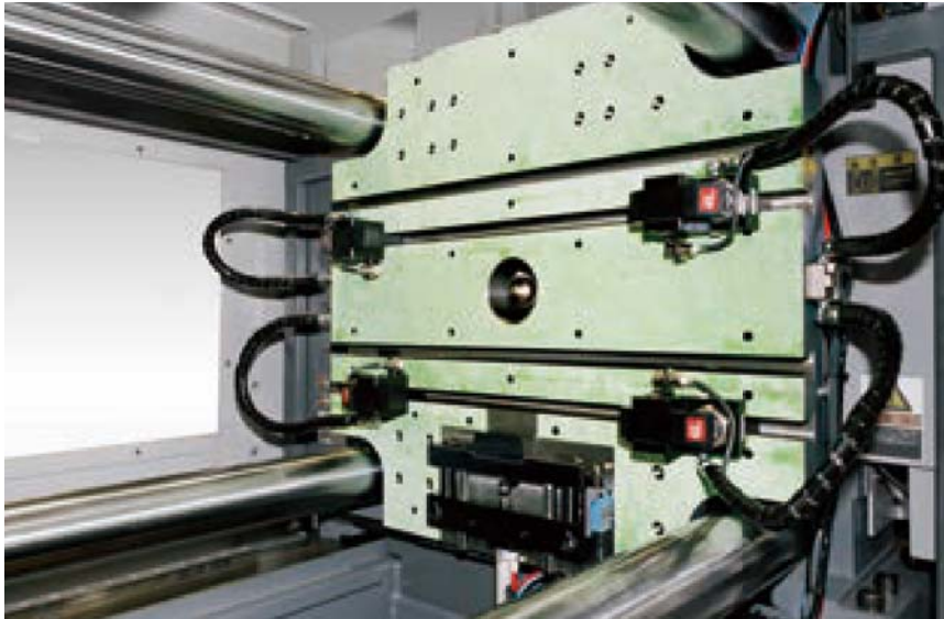
1,800kN (180ton) IMM vertical loading Die setting system & Hydraulic clamp, slidable type TYA040
