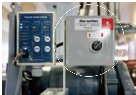
Die setter operation panel
