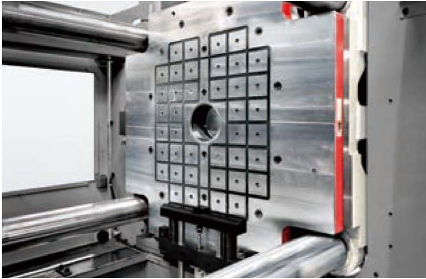
3,500kN (350ton) IMM vertical loading Die setting system & Mag clamp
