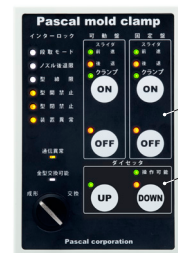
Die setter & Clamp operation panel
