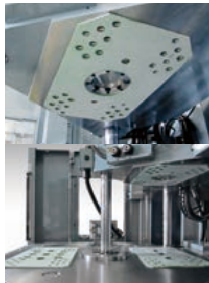
500kN (50ton) Vertical IMM Octagonal locate ring (positioning for upper mold) & Rollers
